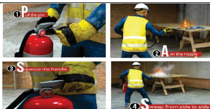
Fig 3.4 Steps to open the seal and safety pin
