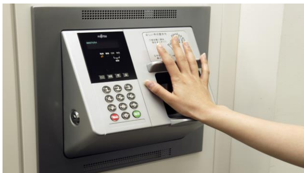
Fig. 2.17 A palm recognition system with palm print scanner
